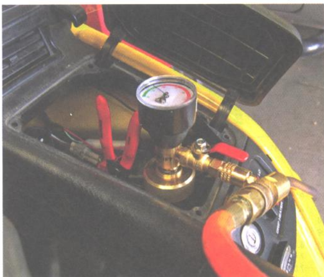
Above: In this image the shop's air hose has been attached to create a vacuum (by venturi effect) to draw out entrapped air.
